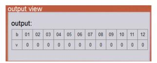
View general output state, also control the output state of general output port. Set 1 means open the corresponding port, set 0 means close the corresponding port.
