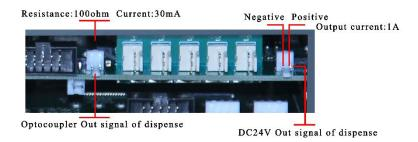
If use optocoupler to output the dispense signal but can't glue or can't stop to glue, we can switch the two edge of the optocoupler output signal.
