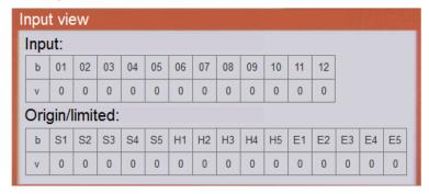
0-12 of "general input" is 12 input states for programmable input port, when check input signal for '1', no input signal for '0'.
