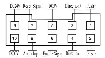
4D2Y Motor axis signal
