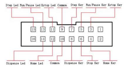
Note: 1. Enable drive indicator LED, connected to the positive terminal (+ 5V), common negative pole
