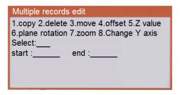
1. **Copy**: as following three pictures, copy 0001-0003 program points to 0005, the third picture is result when the first picture execute the second picture.
